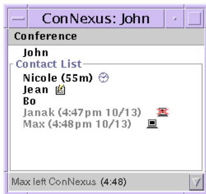
Figure 1. The Contact List provides awareness for a list of users by showing any computer input device idle time and any communication activity indicators for each user.
